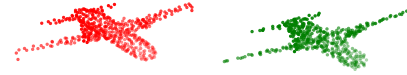
Fig. 2. Point cloud reconstruction from FV representation using a deep decoder. The original (left), and the reconstructed point cloud (right).
